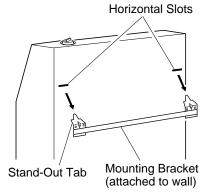
Figure 12 - Mounting Heater Onto Mounting Bracket
